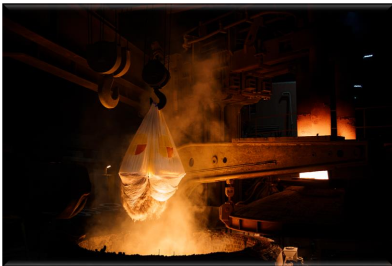
Photo: Adding lime into the Electric Arc Furnace (EAF) by big-bag, SMA Mineral
